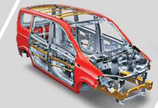
SAFE CAGE STRUCTURE
